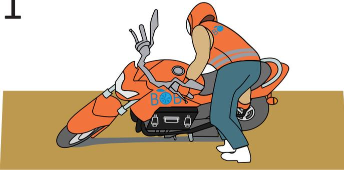
Grab the handlebar with your left hand, and hold the handle with your right hand to support the vehicle.
